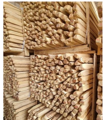
Sawn stakes, debarked, chamfered, Circ. 20-25cm
