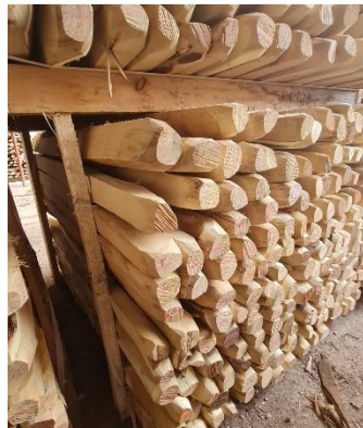
Sawn stakes, debarked, chamfered, Circ. 25-30 cm
