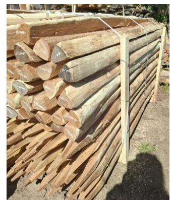
Split stakes, chamfered
