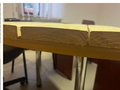
Finger-jointed decking board – convex profile 23 × 118 mm
